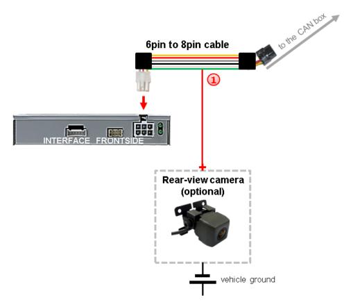
Additionally, the +12V (max. 500mA) power supply for the rear-view camera can be taken from the green wire of the 6pin to 8pin cable.
