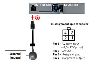
Onnect the female 4pin connector of the keypad to the male 4pin connector of the video-interface.
